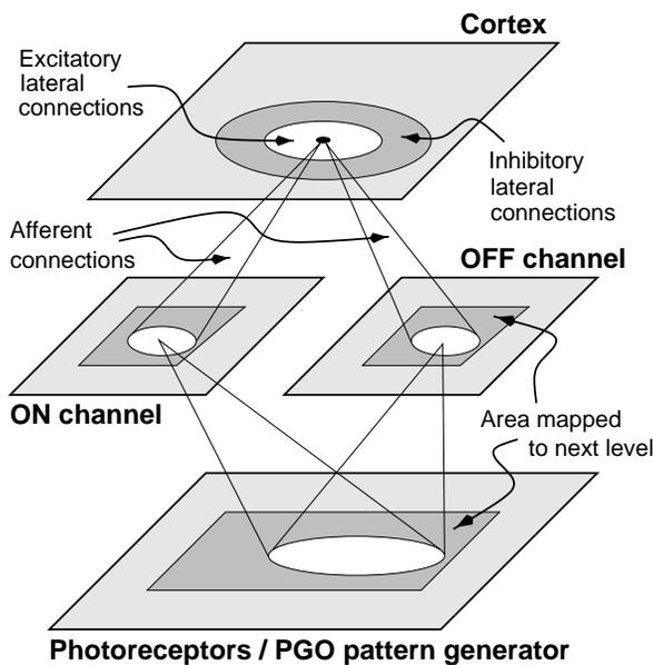
Figure 1: **The CRF-LISSOM model.** A schematic diagram of the CRF-LISSOM network, with connections shown for a single cortical neuron and for an ON-center and OFF-center ganglion cell. Activity propagates from the photoreceptor layer (bottom) up to the cortex and then spreads laterally within the cortex; weights are adapted when the activity settles.
