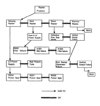
Figure 2-1: A failure-mode hierarchy
