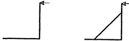
Figure 4. Addition of a beam at points of high deflection in a structure.
